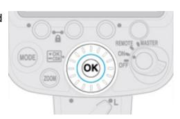
Rotate the selector dial to choose **Version of firmware**, and press the [OK] button.
