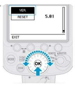
The current firmware version will be displayed. This upgrade can be used with firmware version 5.01.
