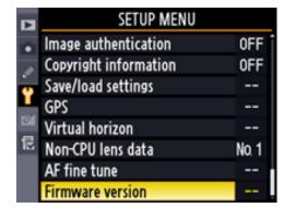
The current versions of the camera and SB-900 firmware will be displayed. Highlight **Update** and press the multi selector to the right.
