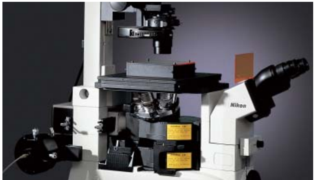
Optional stage risers (70mm) allow the mounting of other equipment such as laser tweezers or a laser unit in addition to an epi-fluorescent attachment without modifying the microscope body.
