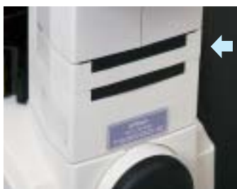
Eye-level riser (as indicated by arrow)
