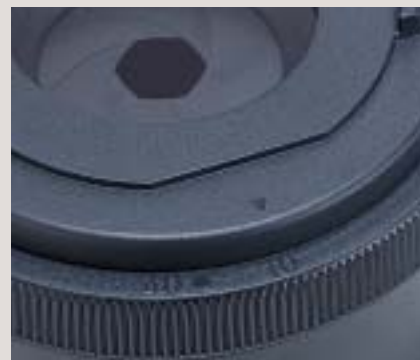
Field diaphragm with position-guide markings.
