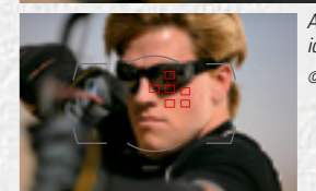
In Single-servo AF, active focus points are highlighted for about one second.
