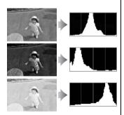
Increasing exposure compensation shifts the distribution of tones to the right, while decreasing exposure compensation shifts the distribution to the left. Histograms can provide a rough idea of overall exposure when bright ambient lighting makes it difficult to see photographs in the monitor.
