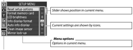
If a ? icon is displayed at the bottom left corner of the monitor, help can be displayed by pressing the ? (९₺) button. A description of the currently selected option or menu will be displayed while the button is pressed. Press  $\triangle$  or  $\nabla$  to scroll through the display.
