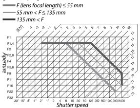
The maximum and minimum values for EV vary with ISO sensitivity; the above graph assumes an ISO sensitivity of ISO 100 equivalent. When matrix metering is used, values over  $16^{1}/_{3}$  EV are reduced to  $16^{1}/_{3}$  EV.
