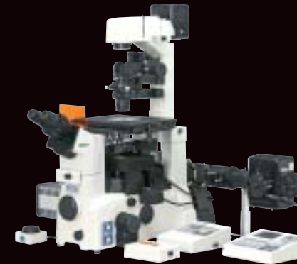
Correction to focus drift caused by expansion/contraction of the plastic dish when reagents are added •PFS on
